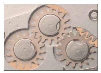
Lubrication of the 3 intermediate driving wheels for ratchtet wheel (HP 1300 Sans Colorant)  $\,$
